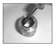
9. The front oil seal (31A) can now be removed by inserting a screwdriver through the rear of the retainer and tapping the seal out through the front of the retainer. Remove any excess old loc-tite from retainer. To replace oil seal, apply a light film of loc-tite around outside edges of seal. Tap seal firmly into the retainer with a wooden dowel making certain that the spring side of the seal is installed first and that the seal sits squarely in the retainer.
